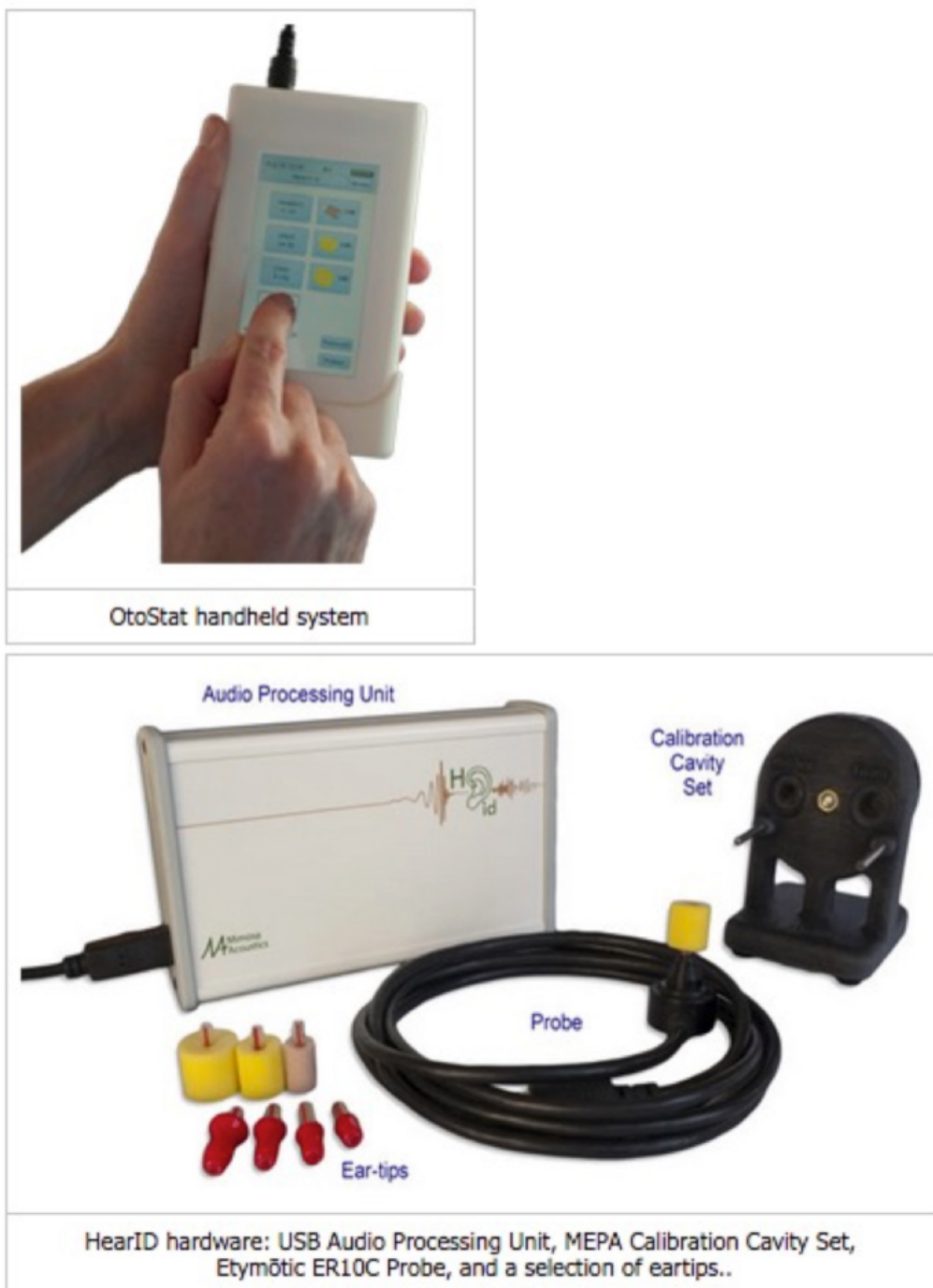
Figure 1. The Mimosa Acoustic devices capable of recording wideband reflectance and OAEs. Data from the Mimosa Acoustics website ( http://www.mimosaacoustics.com ).
